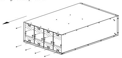
**3** Remove the battery modules from the battery pack.
