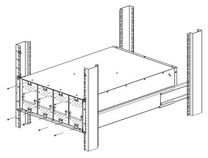
8 Secure the battery compartment door to the battery pack with 6 (M3x8) screws.
