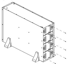
6 Secure the battery compartment door to the battery pack with 6 (M3x8) screws.
