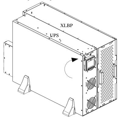
**7** Install the front bezels of both the UPS and the battery pack.
