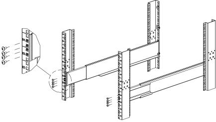
3 Secure the rack-mount brackets to the battery pack with 8 (M4x8) screws.
