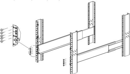
2 Secure the back of rail (SRTGRK2) with 8 (M5x12) screws.
