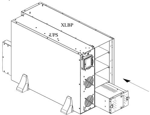
4 Secure the battery modules with 8 (M3x8) screws.
