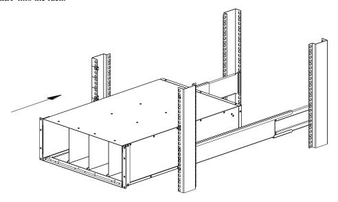
**5** Secure rack-mount brackets to the rack with 4 (M5x12) screws.
