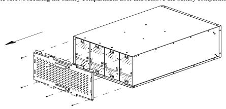
2 Remove the screws securing the battery modules.
