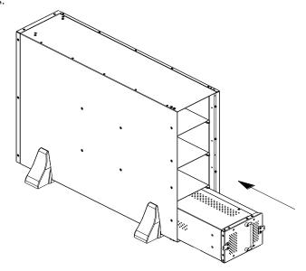
**5** Secure the battery modules with 8 (M3x8) screws.
