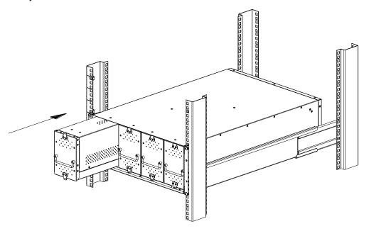
**7** Secure the battery modules with 8 (M3x8) screws.
