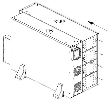
Secure the battery compartment door to the battery pack with 6 (M3x8) screws.
