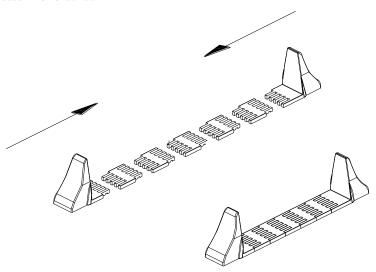
2 Install the UPS module and battery pack on the stabilizer brackets.
